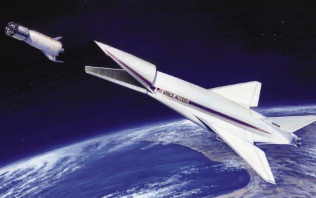
HEAVY SPACE PLANE is being developed by Space Access in Palmdale, Calif. The craft will utilize innovative ejector ramjet engines to accelerate to Mach 6, then switch to rocket engines. Separated stages will individually fly back to the launch strip.
